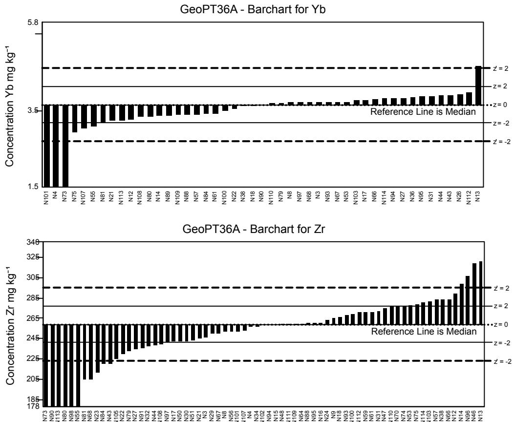
Figure 1: GeoPT36A - Metal-rich sediment, SdAR-M2. Data distribution charts for elements for which values were assigned or provisional values given for guidance. Horizontal lines show the limits for  $-2 < z < 2$  for pure geochemistry labs (solid lines) and  $-2 < z' < 2$  for applied geochemistry labs (pecked lines).
