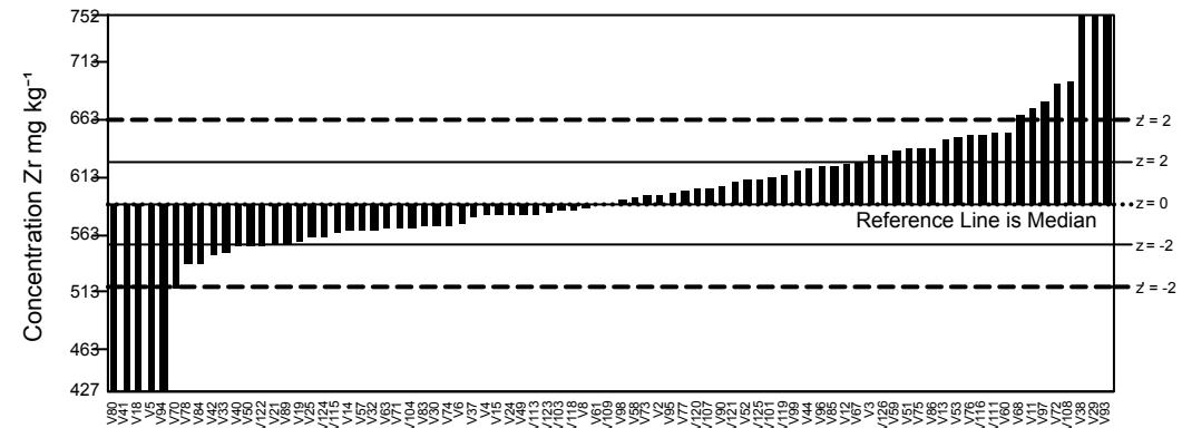
Figure 1: GeoPT39A - Nepheline syenite, MNS-1. Data distribution charts for elements for which values were assigned or provisional values given for guidance. Horizontal lines show the limits for  $-2 < z' < 2$  for pure geochemistry labs (solid lines) and  $-2 < z' < 2$  for applied geochemistry labs (pecked lines).
