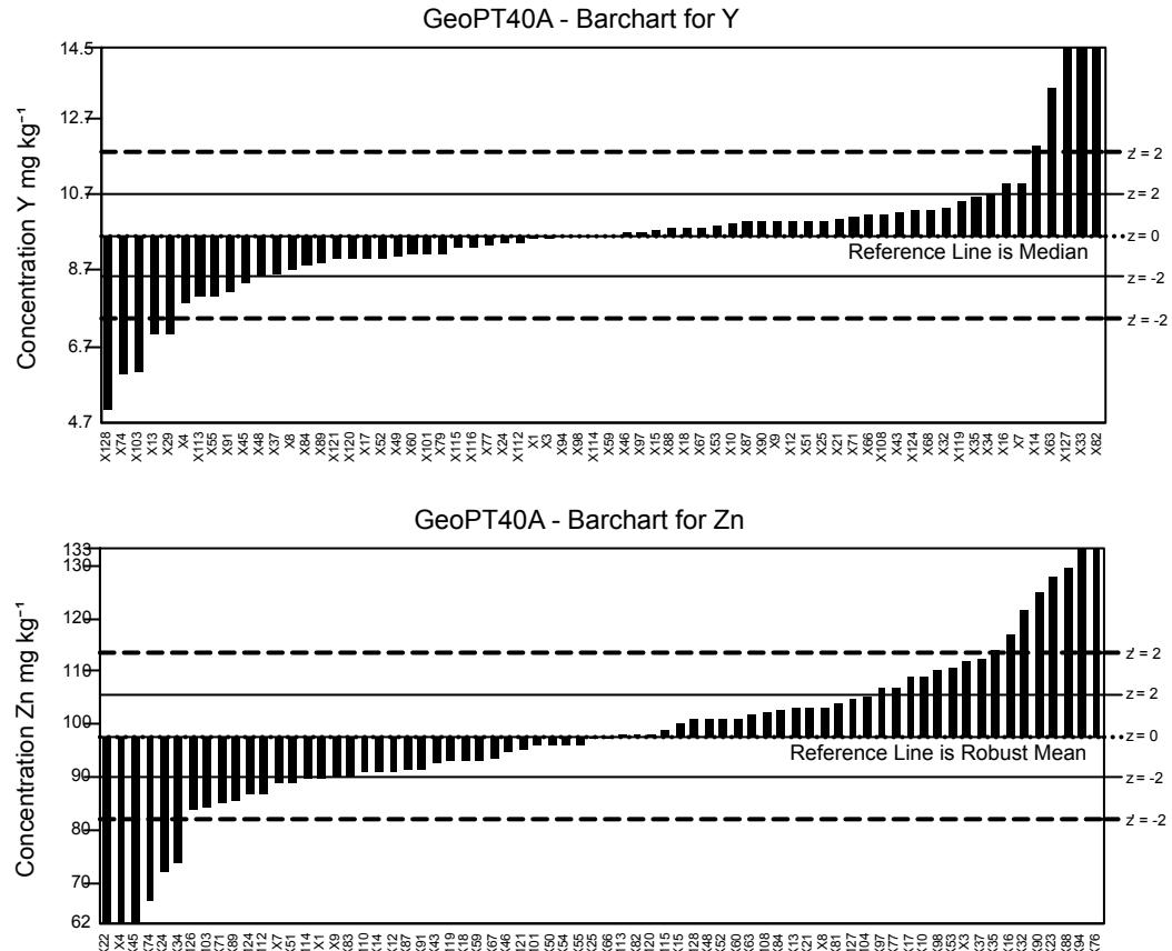
Figure 1: GeoPT40A - Calcareous organic-rich shale, ShTX-1. Data distribution charts for elements for which values were assigned or provisional values given for guidance. Horizontal lines show the limits for  $-2 < z < 2$  for pure geochemistry labs (solid lines) and  $-2 < z' < 2$  for applied geochemistry labs (pecked lines).
