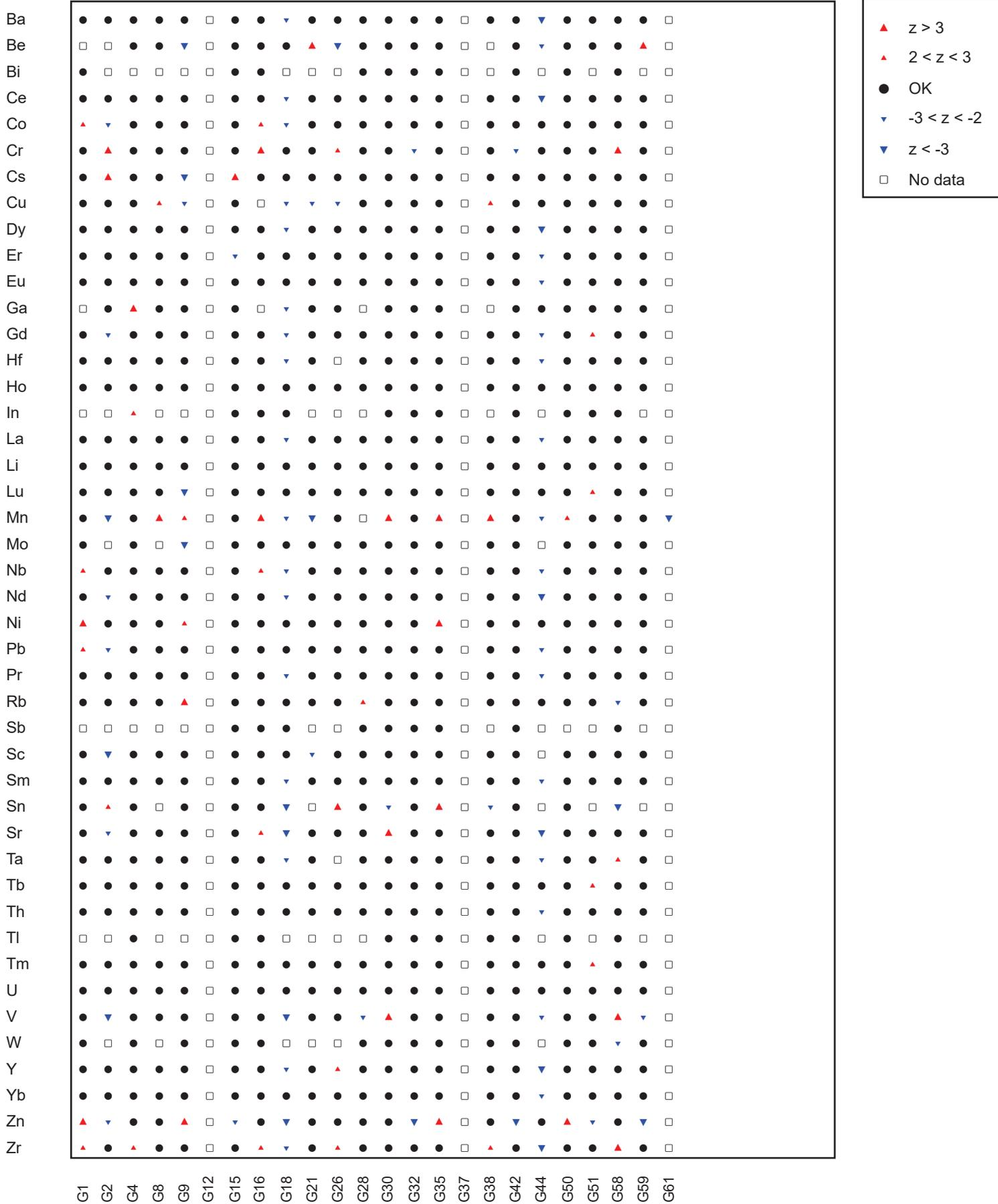
Figure 3: G-Probe 26b - Basalt, KBa-1NP Pellet. Multiple z-score charts for laboratories participating in the G-Probe 26b round. Symbols indicate whether or not an elemental result complies with the  $-2 < z < +2$  criteria (see key).
