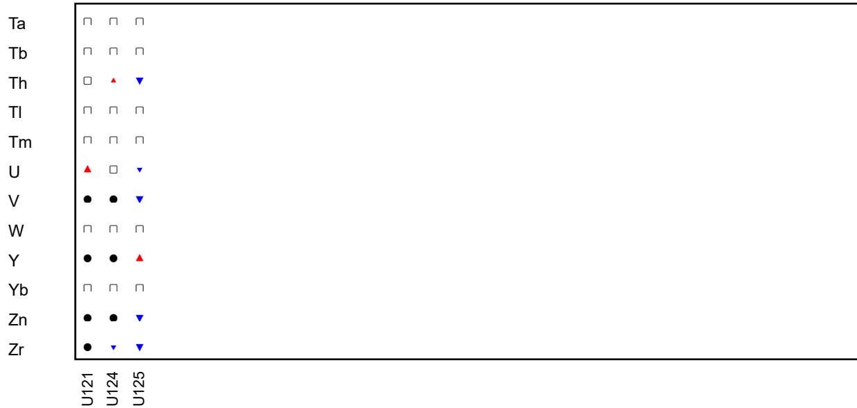
Figure 3: GeoPT54A - Basalt, CSQ-1. Multiple z-score charts for laboratories participating in the GeoPT54 A round. Symbols indicate whether or not an elemental result complies with the -2 < z < +2 criteria (see key).
